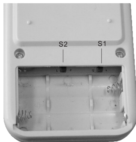
Channel switch position on the remote controller
